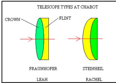
bring two colors into focus. When you look through a refractor, you see a ring of colors around the image of a star or planet. A mirror-type telescope does not have this problem since all colors come into focus. This is one of the many reasons why mirror telescopes are used today. The 20-inch telescope was one of the last large refractors built for a major observatory.
