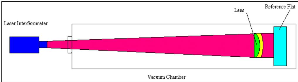
corded. The lens was loaded into the chamber. We used the interferometer as a guide to find the perfect alignment. The crown element was the best choice to rotate. This was done by hand, just like the hour hand on a clock. The fringe changes were observed and recorded at each position. After a few hours of rotating, we discovered a position that gave us the best optical performance.
