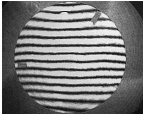
small defects in the lens. The best way to describe this effect is like seeing the hot air rising from a heated road or what makes the stars twinkle at night. The hot air causes waves that distort the image between you and what is ahead. That is why telescopes need to be on high mountain tops or in space. The lens was tested under the best possible conditions.
