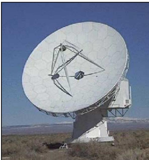
Closeup of a 10-meter radio telescope, part of the millimeter wavelength array. The array consists of six 10.4 meter telescopes with rms surface precision of 35 microns. The aperture efficiencies are 0.70 and 0.45 at 2.7mm and 1.3mm, respectively. The pointing accuracy is about 4" (day and night), except for brief excursions at sunrise and sunset. The halfpower beamwidth is 65" at 100 GHz and scales inversely with frequency.
