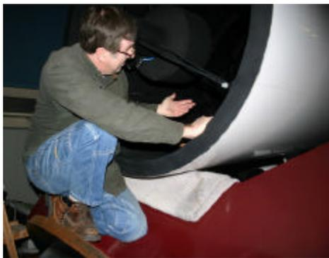
signals between the telescope and the control system chassis, so it was time to trace the cable wires to see where the position sensor signal was being lost. This was especially hard to do because there are intermediate connectors in the long cables, and because we had no wiring diagrams to tell us what pins on the connectors corresponded to which function in the motor housing.
