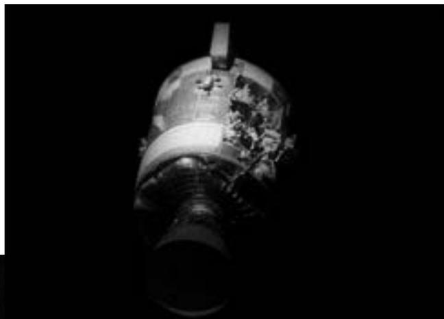
View of the severely damaged Service Module after separation. 17 April 1970. (Source: NASA, image AS13-59-8500, <https://www.hq.nasa.gov/alsj/a13/images13.html>)
